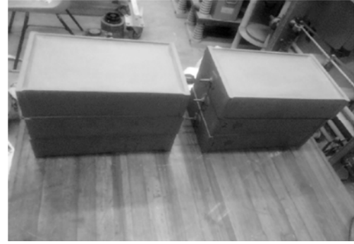
Figure 5. Capacitors of the IVG.
