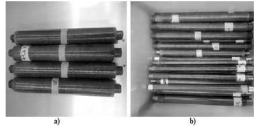
Figure 6. a) Load resistors and b) front and tail resistors.
